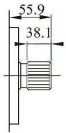
Shaft code 3 SAE C Splined shaft class 1 - J498 b 12/24 dp. -14 teeth 30° pressure angle. Flat root side fit.
